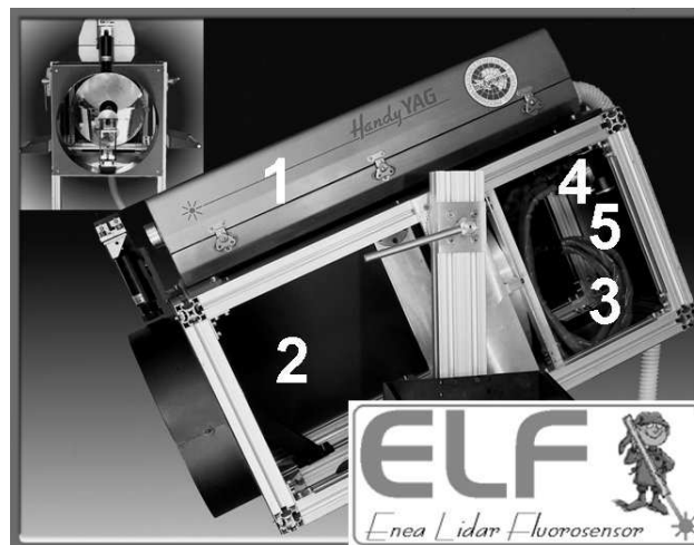
Fig. 5. ELF consists of a transmitter: frequency-tripled Nd:YAG laser (1), a receiver: Cassegrain telescope (2) and a detector: optical fibers (3), bandpass filters (4) and photomultiplier tubes (5).
